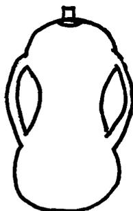
Into this container the substance is given, it should fill about two thirds of the lower half. The Pelican is then set into horse dung up to its "waist line" (or upon some other suitable heating equipment). A thermostatically controlled sand bath or ash bath does very well. The liquid evaporated into the upper portion of the Pelican where it condenses again because of the lower outside temperature, it then flows back through the arms and along the walls.
